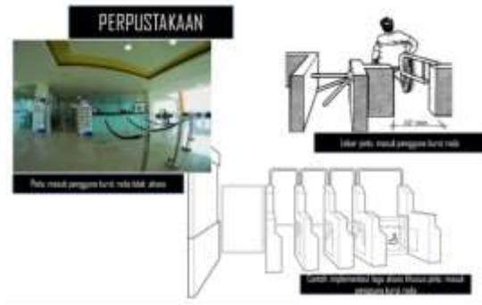
**Fig 10.** Access to reading room entrance of Tower building is difficult to access by wheel users. The proposed design on the detailed picture detailing the size of wheelchair. Sources of detail entrance of counter by regulation of PUPR No. 14/2017. Photo source by Rachmita MH, 2017
